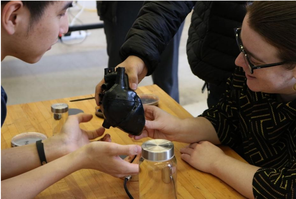
Figure 4. Palpable Pulse 3D-printed pulsing heart, by Jason Zhu, which ‘beat’ as it was held over an electromagnetic base.
