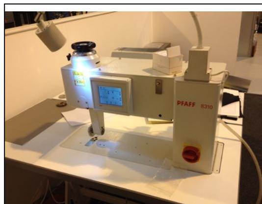
**Figure 11. PFAFF ultrasonic welding equipment**
