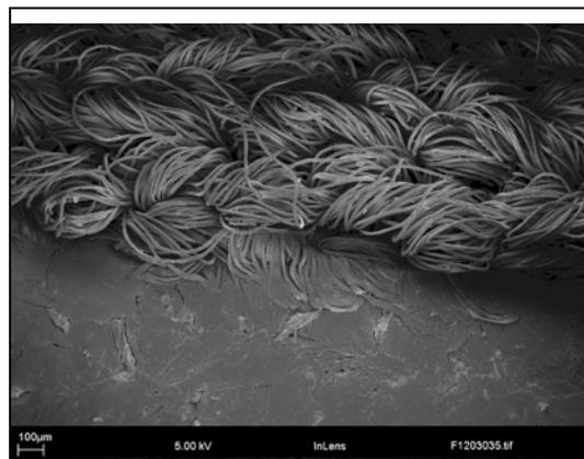
**Figure 18. SEM image of ultrasonic welded knitted textile sample**
