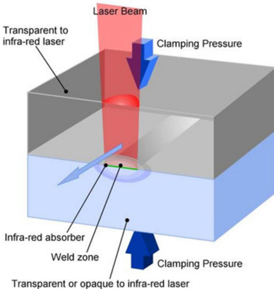
Figure 1. Material configuration for transmission laser welding of textiles
