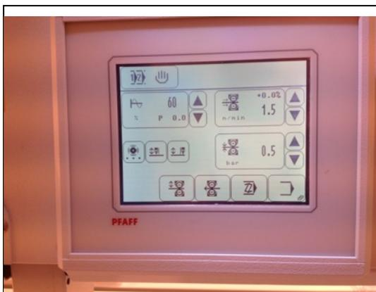
**Figure 10. Digital display of recordable parameters on PFAFF ultrasonic welding equipment**
